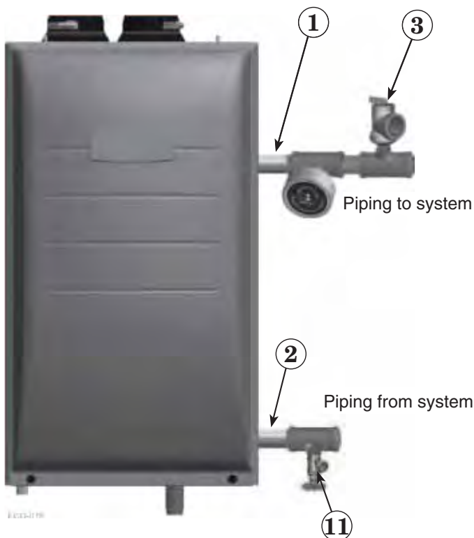
Figure 8 Install pipe fittings for relief valve and pressure/temperature gauge — DO NOT mount relief valve until AFTER hydrostatic testing (see legend below)
