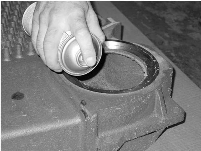
Figure 27 Ceramic Rope Adhesive Application
