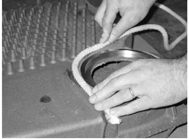
Figure 29 Trimming Ceramic Rope
