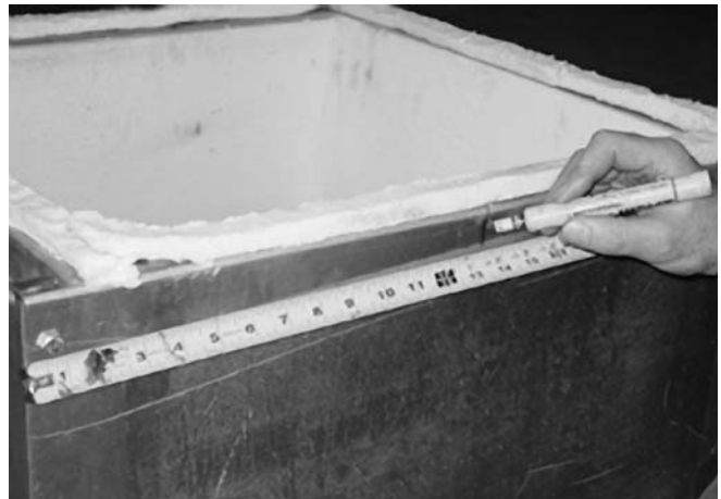
Figure 26A Marking Burner Base Front Midpoint
