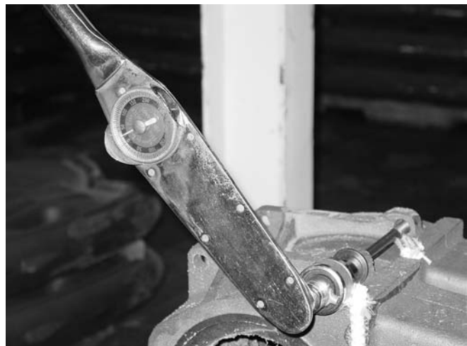
Figure 42 Draw Rod Torquing - 30 ft/lbs, 42 Nm
