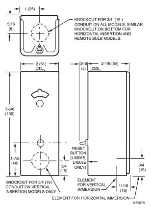
Case Dimensions: 5 5/8 in. high x 2 in. wide x 2 1/8 in. deep (143 mm high x 51 mm wide x 54 mm deep) Maximum Ambient Temperature: 150 F (66 C) Operating Temperature Range: (100 F to 240 F 38 C to 116 C)
