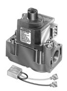
Universal electronic ignition combination gas control for use with direct spark ignition, hot surface ignition or intermittent pilot ignition in 24 Vac, gas-fired appliances, with capacities from 30 to 415 cfh.
