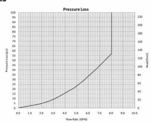
Flow rate is limited to 8.0 GPM.
